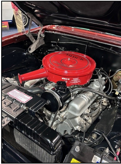
The 425 V-8 was a mid-year option in the 1963 full-size Buicks. This is Jerry Bernard's LeSabre. The silver and red paint scheme is correct for the 1963 425s.
